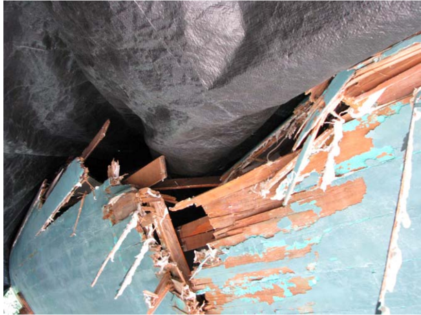
Amorita, starboard side, continuation of gash below waterline, Extending about halfway from the waterline to the keel.
