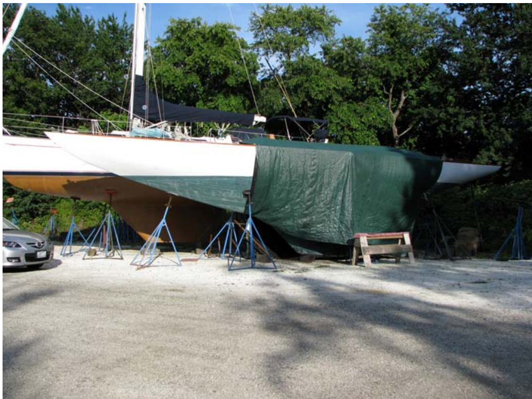
Amorita, port side. Hole extends from bump at sheerline in middle of tarp to about 2/3 of sawhorse length aft, and down to near the waterline.
