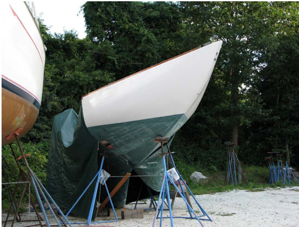
Amorita, starboard side, showing gaping hole in topsides. Gash extends below sag in tarp, shown in next photo. Topsides are also broken aft of hole, where tarp angles inboard.
